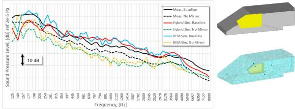
Hybrid method has a great advantage in computation time and delivers results with same accuracy as BEM
