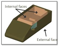
The modular design of the SAE body allows to investigate different configurations of the side mirrors or side glass position.
